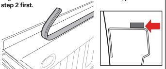
Place the passenger side rail (C) on the truck bed rail with the slotted bracket forward toward the cab/front and facing inside. With the rail firmly placed up to the bulkhead, check that the rail end does not interfere with closing the tailgate. **NOTE**: If the rail end interferes with closing the tailgate and there is a bed liner, trimming a notch in the bed liner with a knife or cutting tool is required - please see step 2A.
