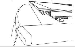
With the cover (A) fully closed, check that the cover panel latches on both sides make proper contact with the side rails. Adjust the cover left to right so that both latches have equal engagement into the side rails.
