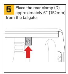
Tighten the clamps (D) starting with the middle, then the front and rear. Always apply downward pressure to the rail when tightening to ensure that the rail sits flush and seals properly. Repeat steps 2 - 6 for the driver side rail (B).
