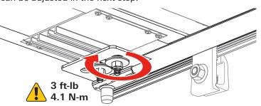
Check for tail panel latch engagement. Check to see that both tail panel latches make proper contact with the side rails. If the tail panel latches do not contact properly, you can manually adjust the latch positions. Remove the small panel screw and slide the end cover off of the latch assembly. Loosen the latch screws (remove and tighten screws by hand only) and slide the latch pall assembly to contact the rail. Check and adjust on both sides. Tighten the screws and replace the cover
