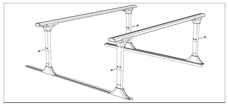
2. Install the Side Bars (#1) to the uprights from the back using 8 Cap Screws (#4), 16 Washers (#6) and 8 Lock Nuts (#5) supplied to accommodate the Side Bars (#1).
