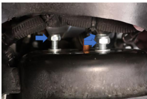
Step 17. Install the 3 17mm bolts provided with the kit along with washers on top of the shock tower. Torque nuts to 52 Ft. Lbs.
