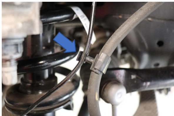
Step1. Detach the speed sensor wire from the brake line clip.
