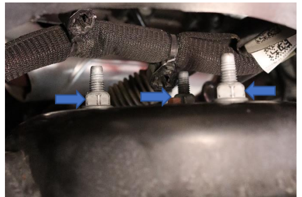
Step 13. Remove the shock absorber and spring assembly upper nuts.
