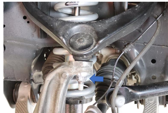
Step 22b. (Torque nut to 26 Ft. Lbs. + 180°)
