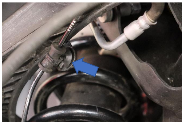
Step 2. Detach the speed sensor wire from the upper control arm bracket.
