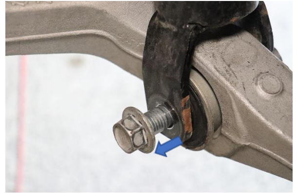
Step 11. Remove the shock assembly lower bolt.
