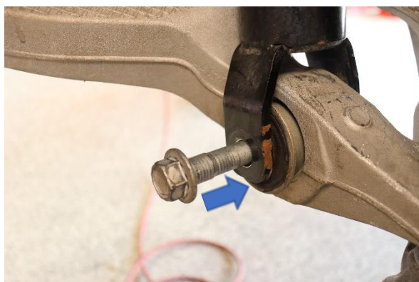
Step 19. Reinsert the lower shock bolt and secure the nut. Torque nut to 124 Ft. Lbs.
