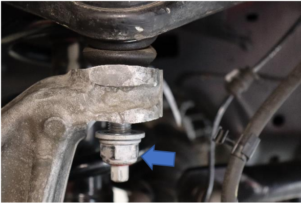
Step 4. Loosen the upper ball joint nut.
