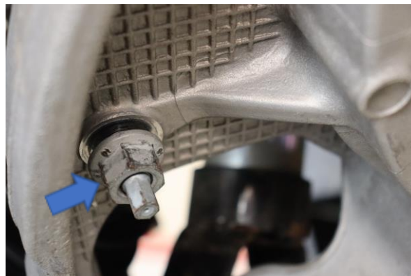
Step 20. Re-insert the stabilizer bar end link and secure the nut at the bottom. Torque nut to 88 Ft. Lbs.
