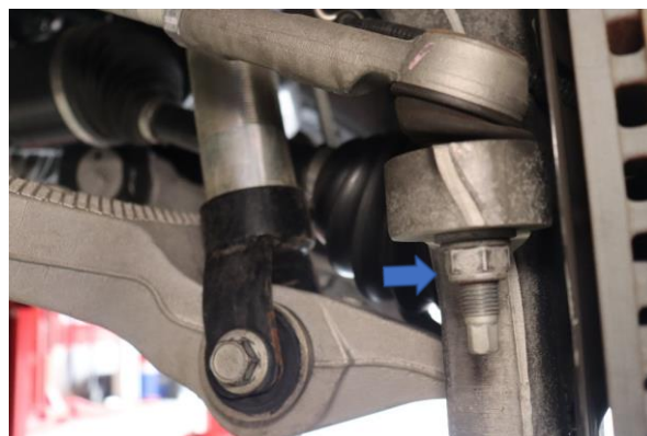
Step 21b. (Torque nut to 38 Ft. Lbs. + 195°)
