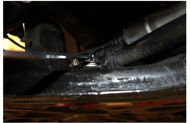
Loosen and remove the bolts securing the sway bar brackets.
