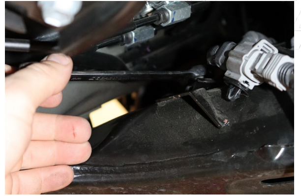
Loosen and remove the bolt securing the bracket to the subframe.
