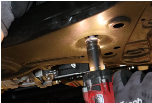
Loosen and remove the bolts securing the steering rack. There is a nut on the other side securing the bolt.
