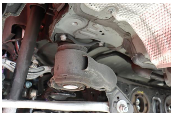
12. Lower the rear subframe.
