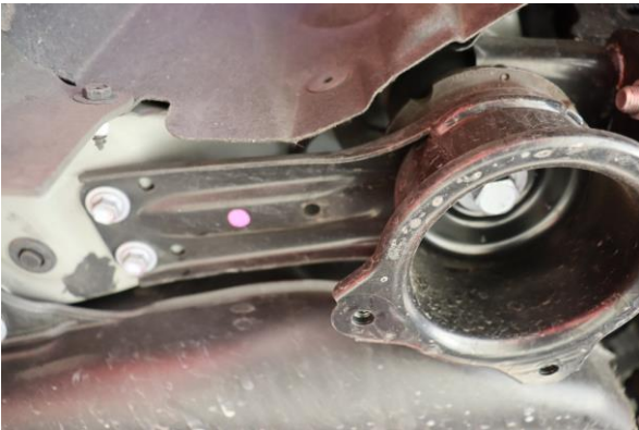
11. Remove the two front bolts and 19mm subframe bolt.
