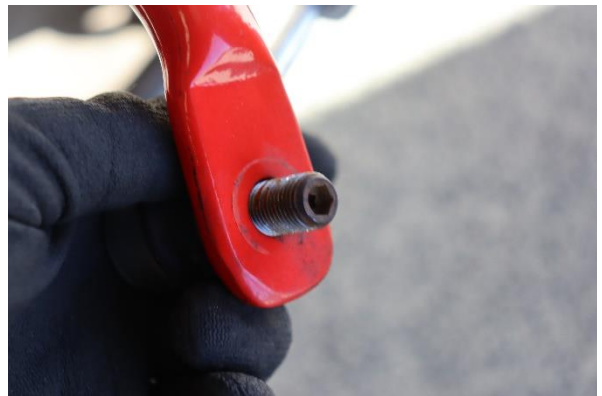
18. Install the OE end link on the Eibach sway bar with the OE 17mm nut.
