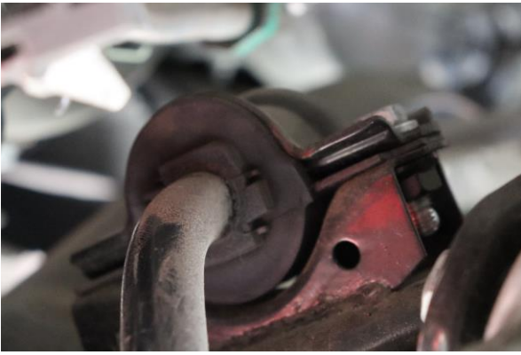
13. Remove the 14 mm bolts for the sway bar bracket. Remove the brackets.
