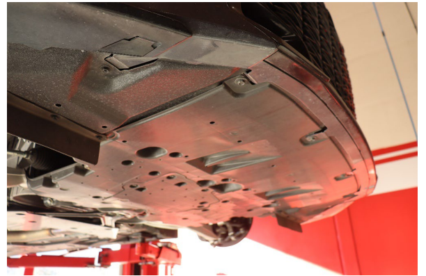
4. Remove the under tray with a 10mm socket and clip pleyer to remove the plastic rivets.
