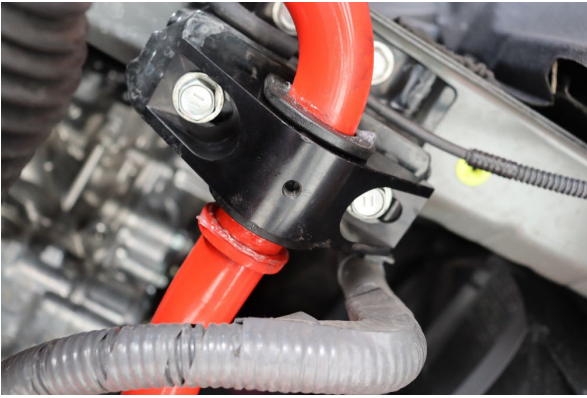
Using the OE bolts mount the Eibach bracket to the subframe.
