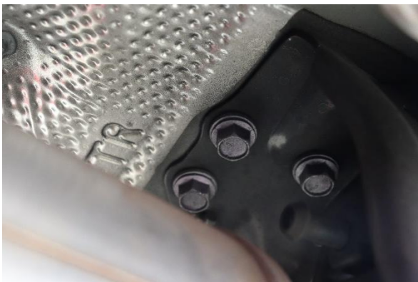
5. Remove the three 17mm bolts that support the muffer.
