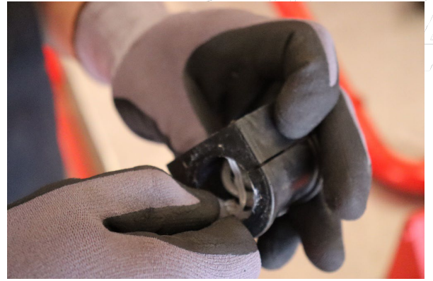
Apply lubricant to the provided Eibach sway bar bushings
