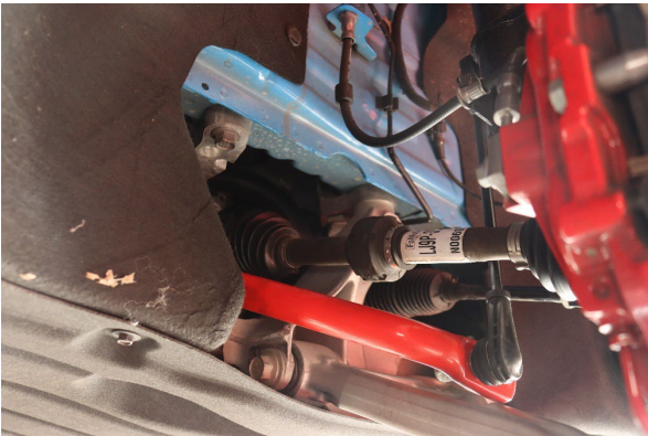
15. Double check all bolts to make sure everything is tight. Reinstall and torque wheel to the proper torque and perform a road test.
