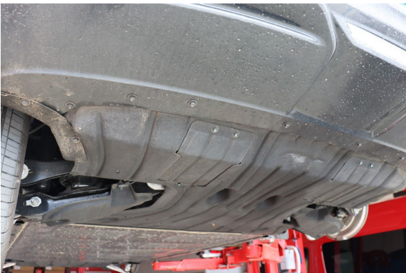
11. Reinstall the OE plastic cover and then road test the vehicle.
