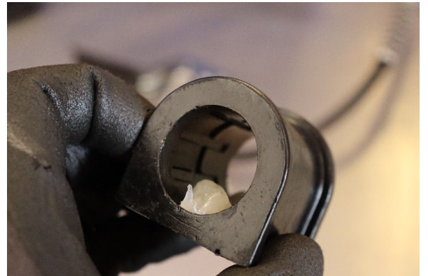
10. Apply the lubricant to the bushing
