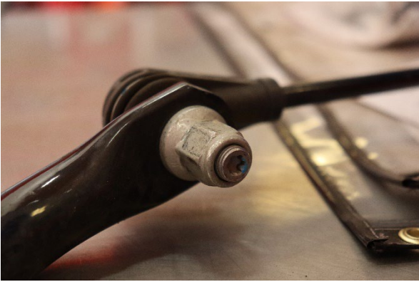
7. Remove the end link from the bar with a 15mm wrench
