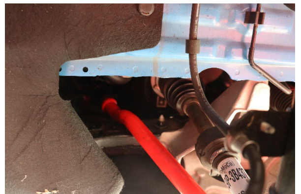
12. Install the bar with the end links and bushings installed.
