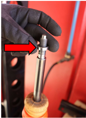
Step 14. Transfer top hat spacer from OE shock.
