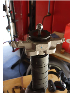
Step 14. Transfer the OE boot, upper shock mount, and spacer/shim. Install 18mm shock shaft nut and tighten to factory specification.
