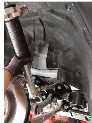
Step 18. Install Eibach shock assembly by lowering onto the lower shock mount and rotating the top of the shock in toward the vehicle.
