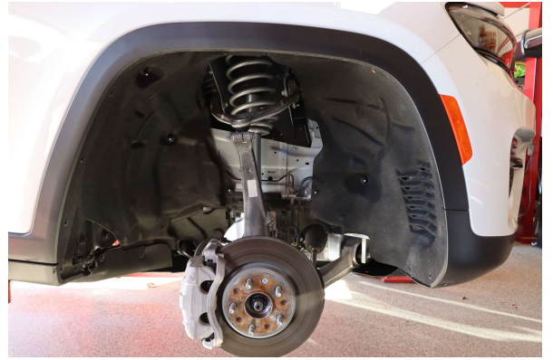
Step 24. Install wheel and tire assembly. Torque 22mm lug nuts to factory specification.
