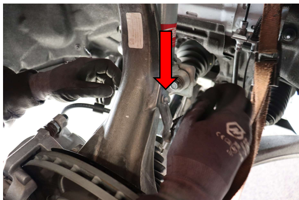
Step 22. Install 10mm bolt securing the wheel speed sensor wiring harness bracket. Tighten to factory specification.
