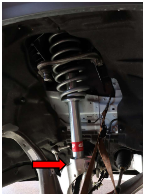
Step 18. Slide lower shock mount up onto lower shock body until fully seated.
