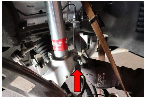
Step 19. Install 15mm lower shock mount nut and bolt. Tighten to factory specification.
