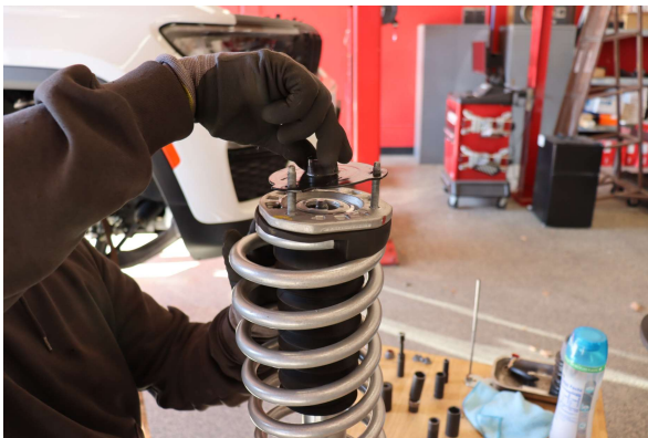
Step 16. Decompress spring assembly and remove from spring compressor. Install OE top hat shim/spacer onto top hat studs.
