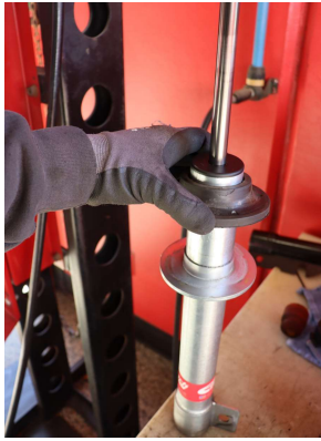
Step 12. Install lower spring perch on shock body. Transfer lower spring isolator from OE shock.
