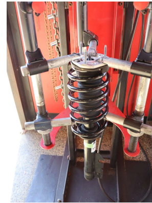
Step 15. Transfer the OE top hat onto the Eibach front spring. Use spring compressor to compress spring and top hat assembly enough that the Eibach shock shaft can be inserted through the bottom of the spring and through the top hat. Tighten shock nut to factory spec.
