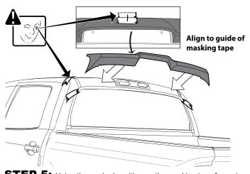
**STEP 5:** Using the marked position on the masking tape from step 3 as a guide, carefully align the cab spoiler to the roof.
