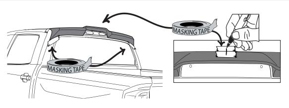
STEP 3: Peel back approximately 50mm (2" in) of tape liner from each of the tape sections and fold liner at 45 degrees to the outside of cab spoiler. Using a blade carefully cut the tape liner in the center of part and peel back at 45 degrees, tape all peeled back sections of tape liner to the outside of cab spoiler using masking tape.
