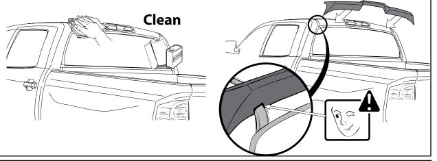
step 2: Align cab spoiler centrally on the roof, ensuring equal spacing around the Center High Mount Stop Light.
