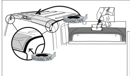
**STEP 3:** Place masking tape on roof aligning the edge of the masking tape to each end on the cab spoiler. Place masking tape centrally on the roof sheet metal and cab spoiler, mark line with a non-permanent pen to assist in positioning.
