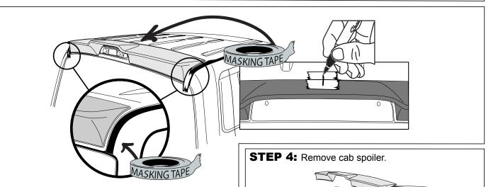
**STEP 3:** Place masking tape on roof aligning the edge of the masking tape to each end on the cab spoiler. Place masking tape centrally on the roof sheet metal and cab spoiler, mark line with a non-permanent pen to assist in positioning.
