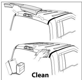
**STEP 1:** Test fit part on vehicle prior to install. Clean the areas on the roof where the cab spoiler will contact the sheet metal using soap and water. A secondary cleaning of isopropyl alcohol can be used, but is not required.
