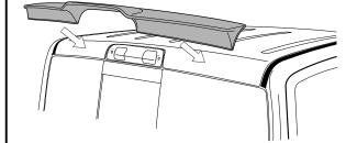
**STEP 1:** Test fit part on vehicle prior to install. Clean the areas on the roof where the cab spoiler will contact the sheet metal using soap and water. A secondary cleaning of isopropyl alcohol can be used, but is not required.
