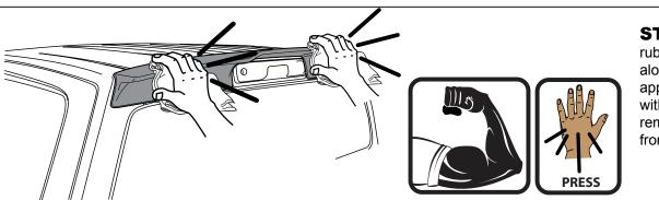
**STEP 8:** Press and rub the cab spoiler down along attachment points approximately 5 times with a dry clean cloth, remove masking tape from roof.
