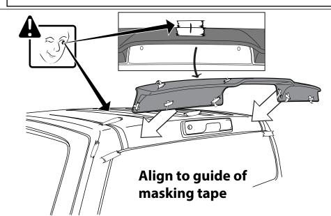
**STEP 6:** Using the marked position on the masking tape from step 3 as a guide, carefully align the cab spoiler to the roof.
