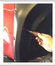
**STEP 5:** Place Fender Flare back on the vehicle into the position of best fit, so the slots in position **A** and **B** (Step: 5) are over the vacant holes in the splash guard areas. Firstly install provided short screw from hardware kit in the vacant slot directly above the slots from position **A** using Philips screwdriver. Re-install the previously removed factory screws in position **B** using a 10mm socket / wrench. Do not fully tighten screws at this stage.
