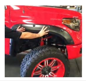
**STEP 9:** If necessary, make minor adjustments to the flare's position to achieve the best fit for your vehicle. When satisfied fully tighten all screw locations, in the above order on which they were installed, to ensure rubber seal is flush neatly against the body.
