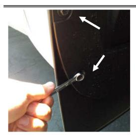
**STEP 3:** Using a 10mm socket / wrench remove the 2 screws from the factory mud flap and retain.
