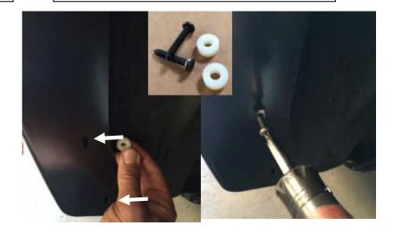
**STEP 6:** Slide the supplied spacers in behind the Fender Flare to fill the gap between the flare and the splash guard/fender. Use a screwdriver or the provided long screws to locate the spacers in line with the factory attachment points. Do not fully tighten screws at this stage.
