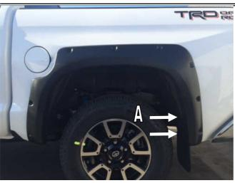
**STEP 11:** Hold Fender Flare onto the vehicle in the position of best fit. Note the slots in the Fender Flare at position **A** that align with the existing screws in the vehicle mud flap. Remove Fender Flare.
