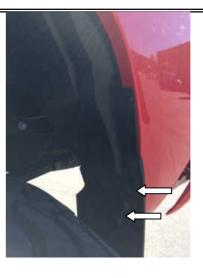
**STEP 12:** Using a 10mm socket / wrench remove the 2 screws from the factory mud flap and retain. These will not be reused in the Fender Flare Installation.
