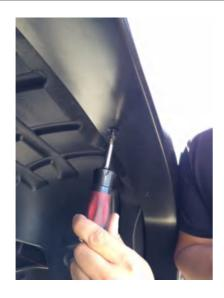
**STEP 13:** Place Fender Flare back on the vehicle into the position of best fit, then install a provided short screw into the top center hole to hold Fender Flare in place. Do not fully tighten screws at this stage.
