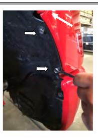
**STEP 4:** Using a 10mm socket / wrench remove the 2 front screws from the inner splash guard area, retain these for later re-install.
