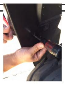
**STEP 15:** At the remaining open 3 slot positions in the Fender Flare, slide the spacer in behind the Fender Flare to fill the gap between the flare and the mud flap / splash guard.
