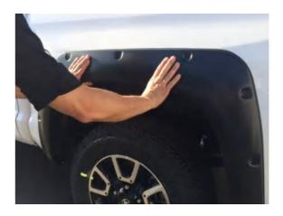
**STEP 18:** If necessary, make minor adjustments to the flare's position to achieve the best fit for your vehicle. When satisfied fully tighten all screw locations, in the above order on which they were installed, to ensure rubber seal is flush neatly against the body.
