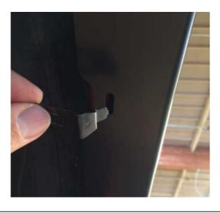
**STEP 8:** Secure attachment clips by sliding clip into Fender Flare slot and using the short screws supplied in the hardware kit to attach screw into existing holes in inner splash guard. Do not fully tighten screws at this stage.
