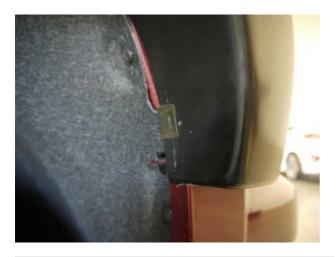
**STEP 7:** To secure the front slot in the Fender Flare to the body, take the black metal clip and slide it over the Fender Flare and the inner wheel arch lip. Position the clip so that the barb in the clip locates in the slot of the Fender Flare. Ensure all fixing points are tight and secure and that the rubber seal is flush neatly against the vehicle body.
