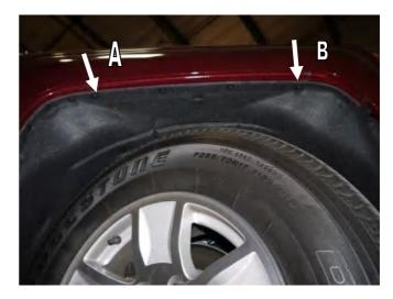
**STEP 2:** Place Fender Flare on the vehicle into the position of best fit. Note where the slots in Fender Flare at positions **A** and **B** align with the existing screws in the vehicle wheel arch. Remove Fender Flare. Remove the existing vehicle screws in location **A** and **B** using #15 Torx head screwdriver. Maintain screws for re-install.
