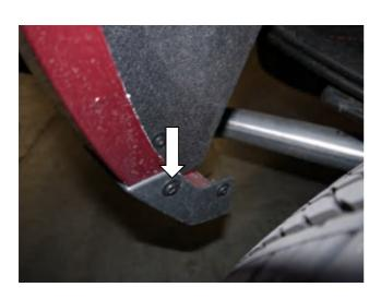
**STEP 9:** Using #15 Torx head screwdriver remove upper screw from the rear factory mudguard. Maintain screws for re-install.
