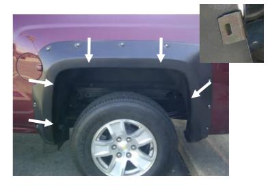
**STEP 10:** To secure the Fender Flare to the body, apply upward tension on Fender Flare to the vehicle fender when installing the black metal clips. Slide the clips over the Fender Flare and the inner wheel arch lip in the five locations shown. Position the clip so that the barb in the clip locates in the slot of the Fender Flare.
