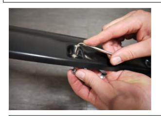
**STEP 1:** Attach the bolts and nuts to each Fender Flare using a 3/16" Allen key or T40 Torx driver and a 10mm wrench/socket. (wrench /socket, Allen / Torx key not supplied). Ensure inside of Fender Flares where the rubber seal is attached is clean, using the alcohol wipes provided. Wipe away any residue with a dry clean cloth.
