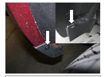
**STEP 14:** Using #15 Torx head screwdriver loosen the top wheel arch facing screw in the front aero spoil. Then remove upper screw from the rear factory mudguard. Maintain screw for re-install.
