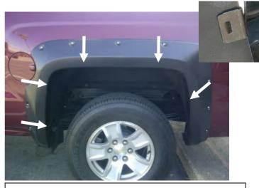
**STEP 15:** Slide the front inner edge of the fender flare behind the aero spoil where previous screw was loosened. To secure, apply upward / inward force toward the vehicle fender. Slide the black metal clips over the Fender Flare and the inner wheel arch lip in the five locations shown. Position so that the barb in the clip locates in the slot of the Fender Flare.
