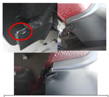
**STEP 16:** Install the "E" shape clip so that the clip slides over the inner sheet metal lip and is in line with the slot in the underside of Fender Flare. To secure the clip to Fender Flare apply inward tension on Fender Flare to the vehicle fender, position the clip so that the barb in the clip locates in the slot of the Fender Flare. Tighten previously loosened #15 torx screw in aero spoil.
