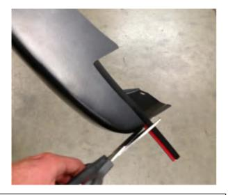
**STEP 12:** Attach rubber seal to the bottom front corner of Fender Flares. Peel back 1" of the adhesive backing and position on the Fender Flare. Attach the seal to the Fender Flare, ensure pressure is used to secure rubber seal to Fender Flare edge. Trim excess rubber seal and discard.
