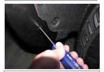
**STEP 9:** Re-install factory screw in the mudguard using #15 Torx head screwdriver through the slot in the Fender Flare. Ensure all fixing points are tight and secure and that the rubber seal is flush neatly against the vehicle body.
