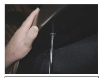
**STEP 8:** Place Fender Flare on the vehicle into the position of best fit so the slots in position **A**, **B** and **C** are over the holes in the front end of large clips. Ensure bottom rear slot in Fender Flare is located over the vacate hole in the factory mudguard. Apply upward tension on Fender Flare to the vehicle fender when Installing the screws and washers provided into the clips in position **A**, **B** and **C** using a Philips head screwdriver.
