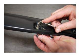
**STEP 10:** Attach the bolts and nuts to each Fender Flare using a 3/16" Allen key or T40 Torx driver and a 10mm wrench/socket. (wrench /socket, Allen / Torx key not supplied). Ensure inside of Fender Flares where the rubber seal is attached is clean, using the alcohol wipes provided. Wipe away any residue with a dry clean cloth.
