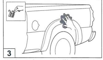
Wash the areas of contact on the vehicle and wipe dry both the vehicle and the Fender Flares with a clean cloth. Ensure inside of Fender Flares where extrusion is attached is clean, use alcohol wipe supplied to clean surface.
