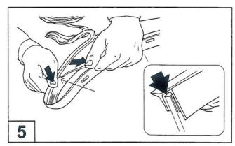
Pulling at right angles to the extrusion, remove the liner from the extrusion in small portions and apply thumb pressure to ensure that it adheres to the Fender Flares.
