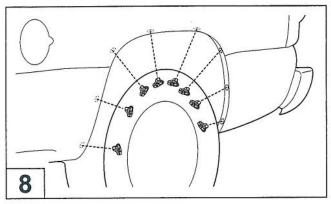
Install the supplied screw plugs into the existing slots as shown.
