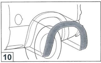
Place the Fender Flare into the position of best fit.
