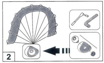
Attach 11 bolts to each Fender Flare using a 3/16" Allen key and a 1/2" wrench/socket. (wrench/socket and Allen key not supplied)
