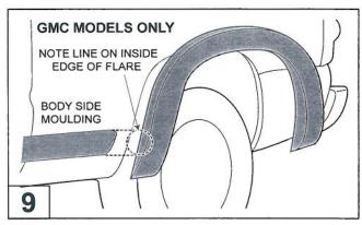
Note the moulded line on the inside edge of the Flender Flare corresponding to the body side moulding. Trim the Fender Flare to this line prior to installing. This is only necessary for GMC Yukon XL models.
