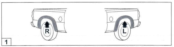
Ensure that both left and right hand Fender Flares suit the profile of the vehicle. Note the areas where the Fender Flares come in contact with the vehicle. **NOTE:** Before fitting Fender Flares remove any mouldings, strips or existing flares from the wheel arch. If there is a body side moulding, mark where the moulding is to be cut, alternatively the Fender Flares can be cut to go around the moulding. Be sure to allow enough room for the extrusion.
