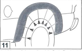
Install the supplied screws through the Fender Flare into the previously installed screw plugs.
