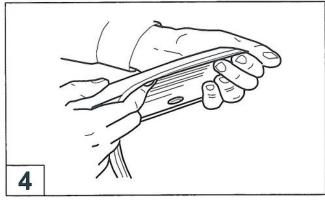
Remove approximately 2" (50mm) of the protective liner from the extrusion. Fit the extrusion to the Fender Flare along the edge that comes in contact with the vehicle's body panel.
