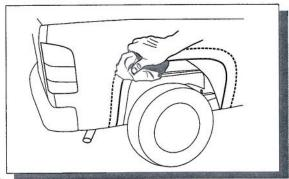
Wash the areas of contact on the vehicle and wipe dry both the vehicle and the Fender Flares with a clean cloth. Ensure inside of Fender Flares where extrusion is attached are clean, use alcohol wipe supplied to clean surface.
