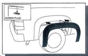
Place the rear Fender Flare onto the vehicle and line up the slot in the Fender Flare with that of the screw plug on the vehicle previously installed.
