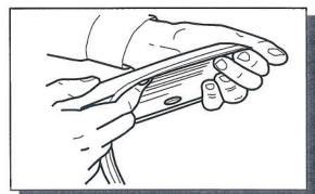
3. Remove approximately 2" (50mm) of the protective liner from the extrusion. Fit the extrusion to the Fender Flares along the edge that comes in contact with the vehicle's body panel.
