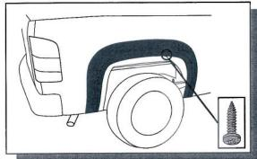
Install the black phillips head screw into the fender and screw plug to secure the Fender Flare. Fit the Fender Flare loosely until the Fender Flare is aligned as desired. When satisfied, tighten the screw fully and ensure extrusion is flush against the body.
