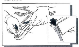
Pulling at right angles to the extrusion, remove the liner from the extrusion in small portions and apply thumb pressure to ensure that it adheres to the Fender Flares.
