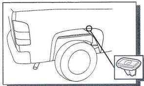
Take the screw plug from the hardware kit and push it into the outside top hole under the wheel arch as shown so it fits tightly.
