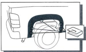
9. To secure the lower part of the Fender Flare to the body, take the black metal clips and slide them over the Fender Flare and inner wheel arch lip. Position clip so that the barb in the clip locates in the slot in the Fender Flare. Ensure all fixing points are secure and that extrusion is flush neatly against the body.
