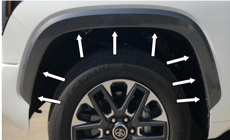
**STEP 2:** Using a 10mm socket / wrench remove factory screw locations (X8) where noted above and retain for re-install.
