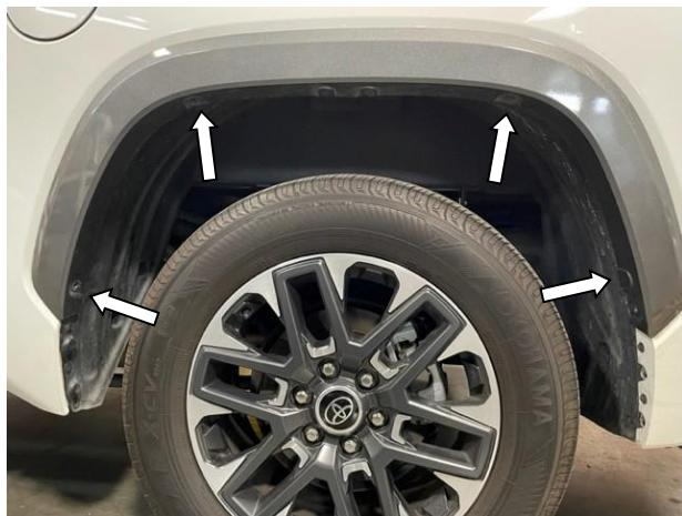
**STEP 7:** Using a 10mm socket / wrench remove factory screw locations (X4) where noted above and retain for re-install.
