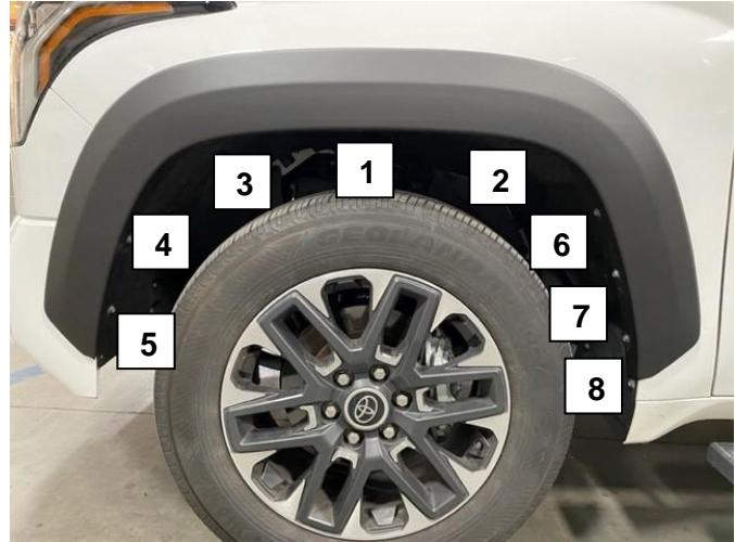
**STEP 6:** Using factory screws that were previously removed begin to loosely screw into slotted hole locations. Once all factory screws have been re-installed, apply pressure and begin to tighten in the order shown above. Ensure rubber seal is sitting flat against vehicle. When satisfied fully tighten all screw locations, in the above order in which they were just installed.
