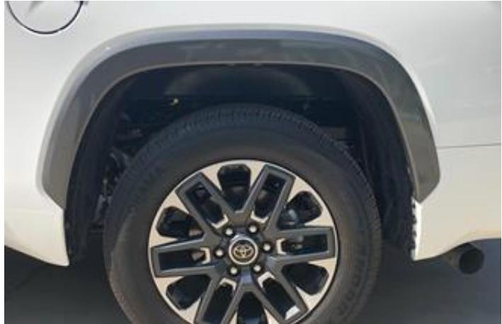
**STEP 8:** Using the alcohol wipes supplied, clean the body area where the Fender Flares will contact vehicle surface. Ensure fender surface is dry prior to install.
