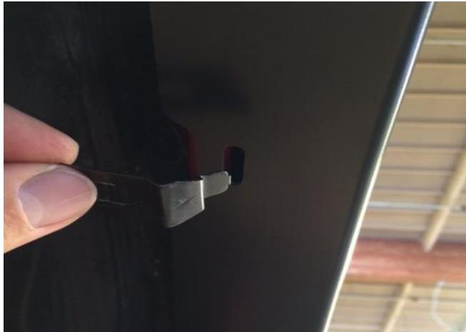
**STEP 5:** Secure attachment clips by sliding clip into Fender Flare slot. Using the factory screws that were previously removed, attach the clips into corresponding existing holes in upper inner splashguard. Do not fully tighten screws at this stage.
