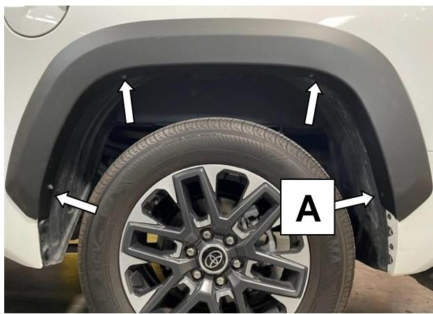
**STEP 9:** Hold Fender Flare on the vehicle in the position of best fit. Note where all the slots in the Fender Flare align with existing mounting holes on the vehicle. Make note of position (A) as it will require hardware in the kit supplied. All remaining positions will re-use factory screws.
