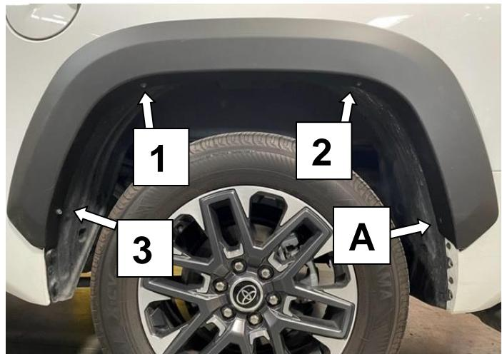
**STEP 10:** Begin to loosely install factory screws into the corresponding factory attachment points. Once all factory screws have been re-installed, begin to fasten in the order shown above. Do not fully tighten screws at this time.
