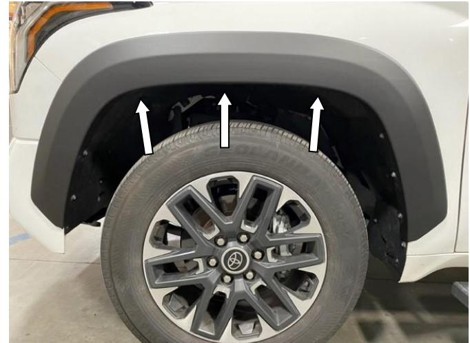
**STEP 3:** Clean the body areas where the Fender Flares will contact the vehicle surface. Ensure fenders are dry prior to install.
