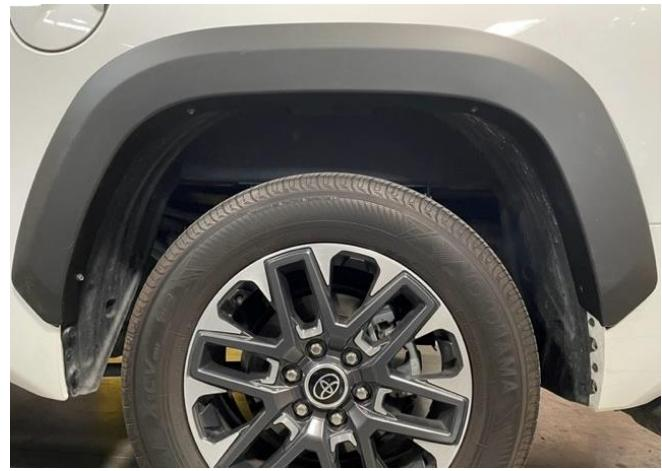
**STEP 11: POSITION (A)** - Ready the spacers (and long screw) to go in behind the Fender Flare to fill the gap between the flare and the vehicle.
