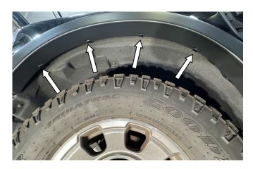
**STEP 9:** Ensure all fixing points are tight and secure and that the extrusion is flush neatly against the vehicle body. Repeat install steps for the opposite side.
