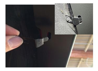
**STEP 7:** Slip end of clip into slotted hole of the fender flare, per image above. Using factory screws that were previously removed, begin to loosely screw into slotted hole locations. Once all factory screws have been reinstalled, apply pressure and begin to tighten in the order shown above. Ensure rubber seal is sitting flat against vehicle. When satisfied fully tighten all screw locations, in the above order in which they were just installed.
