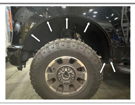
STEP 5: Remove factory screw locations (X6) where noted above and retain for re-install.
