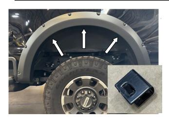
**STEP 15:** Note where the slot locations are in the Fender Flare. Using the U-CLIP supplied (without the "X" mark) begin to clip the fender flare to the wheel well lip where specified above. Be sure the clip engages to the slot of the fender flare.
