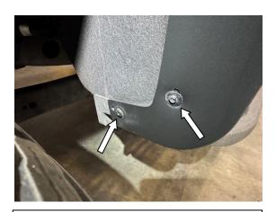
**STEP 8:** loosely re-install factory screws at the rear of the front wheel well area.
