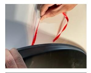
**STEP 10:** Starting at one end of the Fender Flare, carefully remove tape liner from the rubber seal a few inches at a time. Ensure rubber seal is not tucking into flare and sits flush neatly against the fender body. Apply forward pressure to adhere the rubber seal along the edge of entire length of Fender Flare once rubber seal liner is removed.
