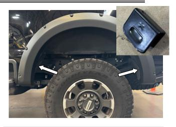
**STEP 16:** Place Fender Flare on the vehicle into the position of best fit. Note where the slots in Fender Flare. Using the U-CLIP supplied (with the "X" mark) begin to clip the fender flare to the wheel well lip where specified above. Be sure the clip engages to the slot of the fender flare
