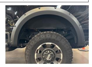
**STEP 14:** Hold Fender Flare on the vehicle in the position of best fit. Remove fender flare and peel back 2" of the red tape liner at both ends.
