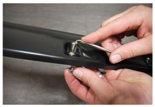
**STEP 11:** Attach the bolts and nuts to each Fender Flare using 3/16" Allen key/Trox and a 1/2" wrench/socket. wrench/socket. (wrench /socket and Allen key not supplied). Ensure inside of Fender Flares where the rubber seal is attached is clean, using the alcohol wipes provided. Wipe away any residue with a dry clean cloth.
