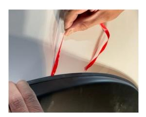
**STEP 10:** Starting at one end of the Fender Flare, carefully remove tape liner from the rubber seal a few inches at a time. Ensure rubber seal is not tucking into flare and sits flush neatly against the fender body. Apply forward pressure to adhere the rubber seal along the edge of entire length of Fender Flare once rubber seal liner is removed.
