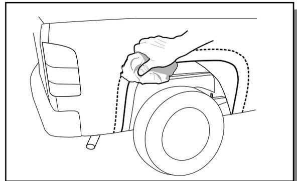
3. Wash the areas of contact on the vehicle and wipe dry both the vehicle and the Fender Flares with a clean cloth. Ensure inside of Fender Flares where extrusion is attached are clean, use alcohol wipe supplied to clean surface.
