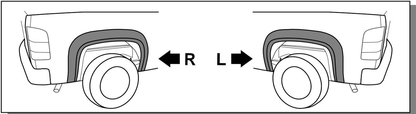
1. Ensure that both left and right hand Fender Flares suit the profile of the vehicle. Note the areas where the Fender Flares come in contact with the vehicle. **NOTE:** Before fitting Fender Flares remove any mouldings, strips or existing flares from the wheel arch. If there is a body side moulding, mark where the moulding is to be cut, alternatively the Fender Flares can be cut to go around the moulding. Be sure to allow enough room for the extrusion.
