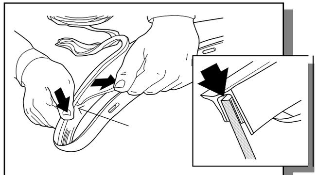
5. Pulling at right angles to the extrusion, remove the liner from the extrusion in small portions and apply thumb pressure to ensure that it adheres to the Fender Flares.
