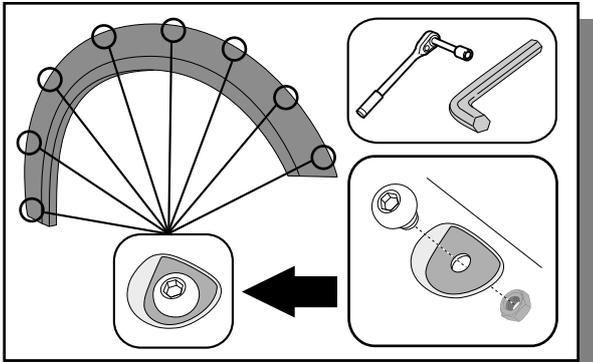
2. Attach bolts to each Fender Flare using a 3/16" Allen key and a 1/2" wrench/socket.
