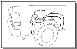
Wash the areas of contact on the vehicle and wipe dry both the vehicle and the Fender Flares with a clean cloth. Ensure inside of Fender Flares where extrusion is attached are clean, use alcohol wipe supplied to clean surface.
