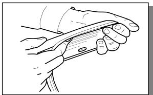
4. Remove approximately 2" (50mm) of the protective liner from the extrusion. Fit the extrusion to the Fender Flares along the edge that comes in contact with the vehicle's body panel, ensuring the double sided tape is being adhered to the inside surface of the fender flare.
