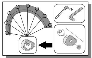
Attach bolts to each Fender Flare using a 3/16" Allen key and a 1/2" wrench/socket.
