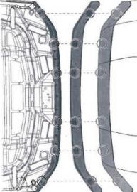
At the previously noted scrivet locations carefully remove the scrivets attaching the hood seal and discard.
