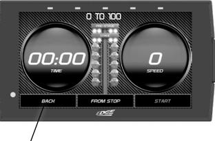
NOTE: Once the speed has been reached, the test will stop and the results will be displayed. A digital drag slip will be created providing run information such as reaction time, speed at specific distances, and other useful information.
