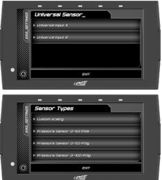
the sensor manufacturer. If it's a resistive based sensor, you can toggle from *Voltage* to *Resistance*. Doing this will allow you to also select the
