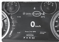
**STEP 5** - With the desired units displayed, press the RES+ button to select the Unit.
