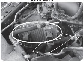
Cut the zip ties that fasten each connector harness to the metal bracket.
