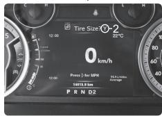
**STEP 1** - With the ignition in the RUN position (Do Not Start), press and hold the CANC (Cancel) button for approximately 5 seconds. *The option to modify the Tire Size is displayed.*
