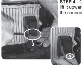
**STEP 4** - Once the lever is released, lift it upward until it stops. Disconnect the connector from the ECM.
