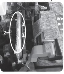
**STEP 3** - Use a flat head screw driver to press the lever lock towards the ECM. Gently lift up on the lever until you feel the lever release.
