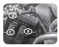
**Note:** The pulsar PCM assembly will now be permanently mounted on an angle from the original bracket.
