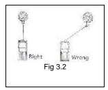
⚠Do not winch from an acute angle as the wire rope will pile up on one side of the drum causing damage to wire rope and the winch. Fig 3.2
