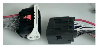
**STEP 8** - Connect the CAT6 harness to both ends of the PCM connector.
