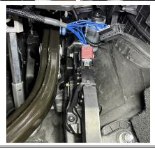
**STEP 10 -** Plug the OBDII connection to the vehicle's OBDII port. Please note the location of the OBDII port on your vehicle may be different from the pictures shown below.
