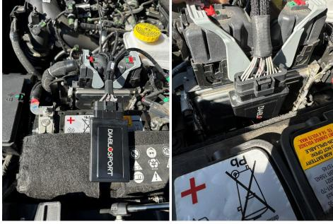
**STEP 14** - Secure the CAT6 harness away from any moving parts or anything that may get hot. Reconnect both batteries and replace the engine cover to finish the installation.
