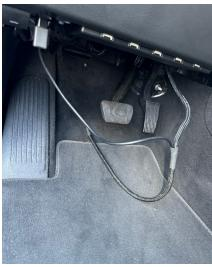
**STEP 11 -** Locate the grommet for the hood latch release cable on the firewall next to the steering column. Using a precision knife, cut a slit into the grommet and pass the Access Link connector from the cabin to the engine bay.
