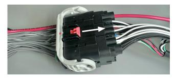
**STEP 7b** - Push down on the release tab shown below to unlock the rotating latch.
