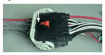
**STEP 7c** - Rotate the latch 180 degrees and pull the connector apart to disconnect.
