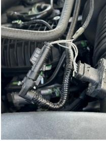
**STEP 5 -** Locate the MAP (Manifold Absolute Pressure) sensor on the intake manifold. Disconnect it by pulling out the white lock tab and then squeezing the same white lock tab, pull to release the connector.
