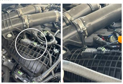
**STEP 6** - Connect both ends of the CAT6 harness to the MAP sensor and the MAP sensor harness.
