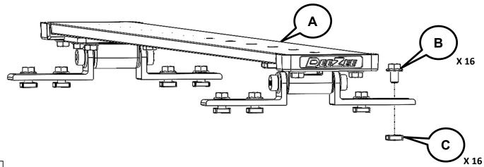
2 Slide hinge assembly onto cross rails on the tonneau cover. Leave hardware loose.
