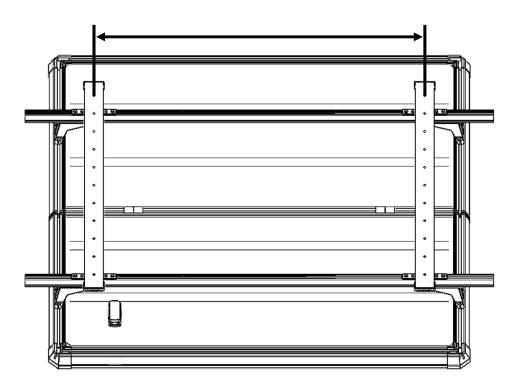
4 Use bolts (D) and nuts (E) through sliding track, if necessary, to mount other accessories.
