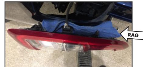
**NOTE:** The taillight may contain a blind spot sensor. Detaching the light and turning the ignition to "ON" may affect this sensor. Do NOT disconnect the taillight and turn the key.
