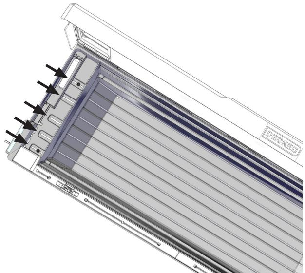
NOTE: Outermost clamp locations vary per vehicle depending on the topology of the bed rails.
