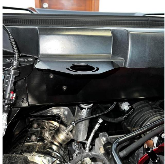
2. Locate the two bolt holes next to the passenger side shock tower. Use the provided hex bolts and a 4mm Allen Wrench to secure the bracket in place.
