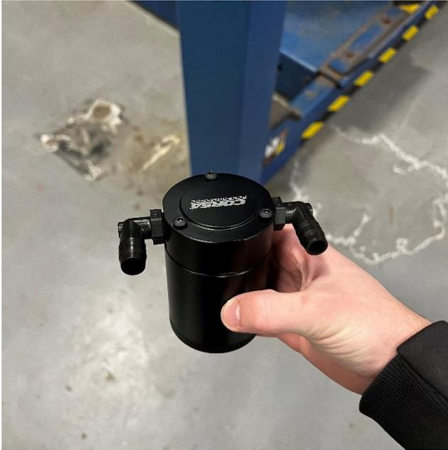
1. Install 3/8" NPT fittings to catch can using an 11/16" wrench. **IMPORTANT:** Corsa recommends using thread sealant or PTFE tape on barbed fittings and bottom drain plug to prevent any leaks.
