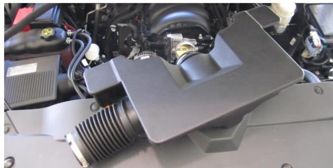
5. Remove the factory resonator box.
