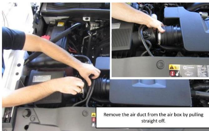
3. Remove the air duct from the air box by pulling straight off.
