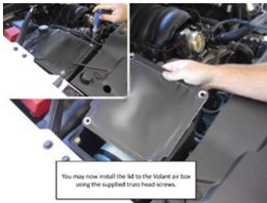
**7.** You may now install the lid to the CORSA air box using the supplied truss head screws.
