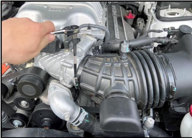
6. Using a 8mm Socket & Ratchet or Wrench, loosen the clamp on the Factory Duct at the Throttle Body. Then remove the Factory Duct and Airbox as one piece. Set these parts aside. Parts will be removed and reused starting in Removal Step 12 and in Install Steps 8 and 11.
