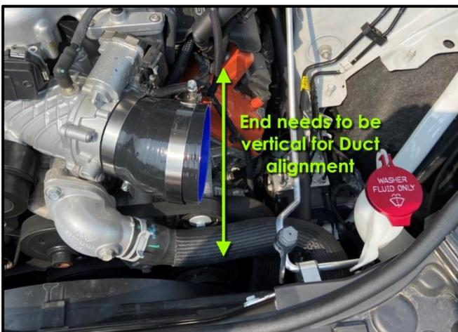
6. Locate the 4.0in to 4.5in Angled Reducer, 4.375in T-Bolt Clamp, and 4.75in T-Bolt Clamp. Assemble the 4.375in T-Bolt Clamp over the smaller end of the Angled Reducer and the 4.75in T-Bolt Clamp over the larger end. Rotate the Angled Reducer so the larger end is vertical. Snug the smaller T-Bolt Clamp with a 10mm Socket & Ratchet or Wrench but do not fully tighten at this time. Leave the large T-Bolt Clamp loose at this time.
