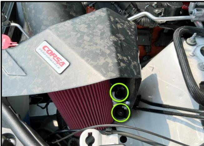
14. Install the CORSA Duct, Filter, and Heat Shield into the vehicle. Insert the Duct into the Angled Reducer first. Next, rotate the Heat Shield and Duct into position and align the Factory Grommets with the Mounting Studs on the Inner Fender area. Ensure the front tab of Heat Shield goes in front of the Washer Fluid Reservoir.
