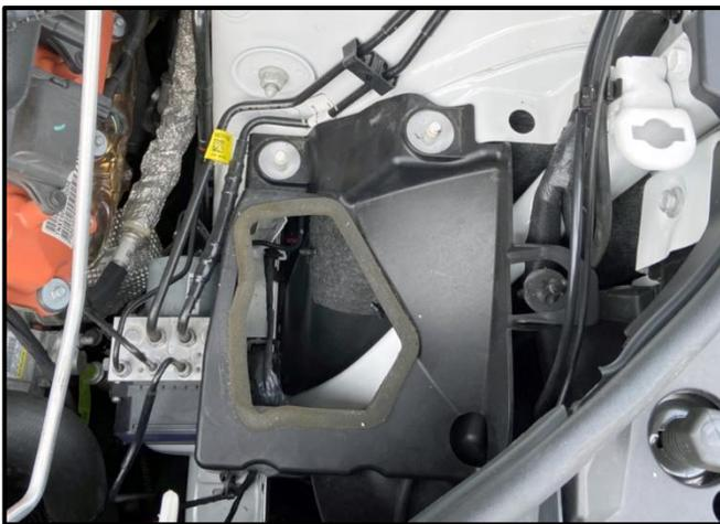
7. After removing the Factory Air Box, remove the Factory Mounting Bracket. This will not be reused.
