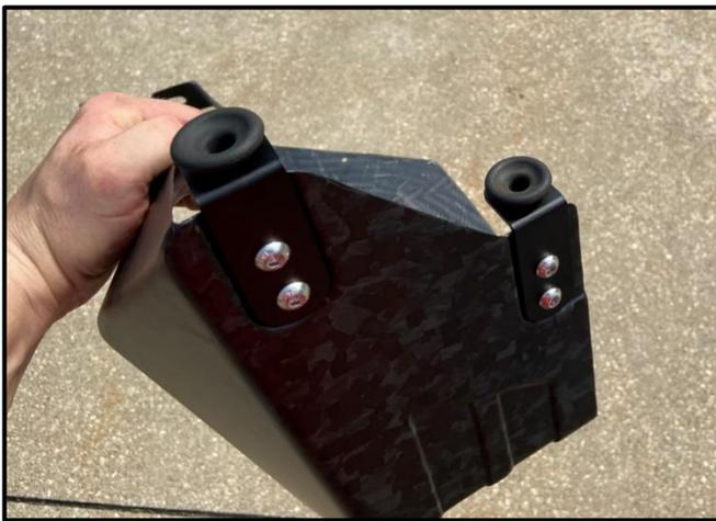
11. Locate the Factory Grommets from Install Step 13 and insert the Grommets into the hole on the bottom of the Brackets as shown.
