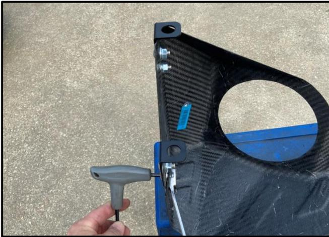
10. Locate the CORSA Carbon Fiber Heat Shield, 2 90deg Brackets, and M8 Hardware. Use a 5mm Hex Driver and 13mm Socket & Ratchet or Wrench to tighten the Hardware.
