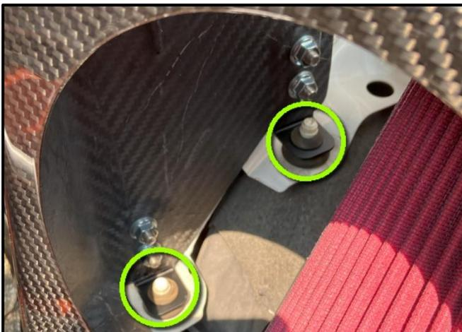
15. Push the grommets onto the Mounting Studs until they are secured. The duct and filter are removed for clarity in the image.
