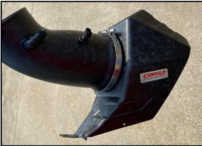
13. Locate 6.50in T-Bolt Clamp. Remove the Nut from the T-Bolt Clamp. Open the T-Bolt Clamp and wrap it around the open end of the Air Filter. Next, close the T-Bolt Clamp and thread the Nut back onto the Stud of the T-Bolt Clamp. Snug the T-Bolt Clamp with a 10mm Socket & Ratchet or Wrench, securing the Duct and Filter.
