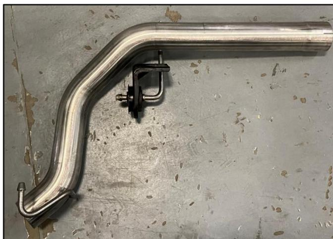
2. Locate the CORSA Front of Tire Tail Pipe. Install the Factory Grommet from Step 1 on to the Front Hanger, as shown. Make sure to orient the Factory Grommet as it was on the Factory exhaust.
