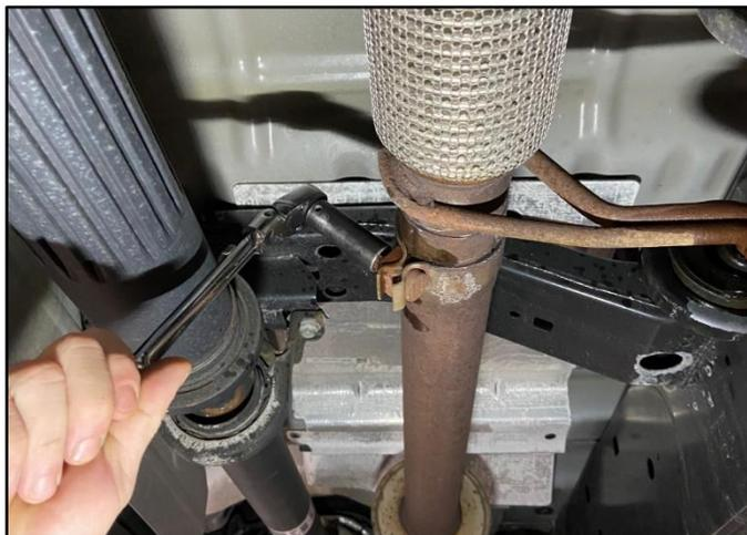
1. Use a 15mm Socket & Ratchet or Wrench to loosen the Stock Clamp, connecting the Front Section and Rear Section of the Stock exhaust.
