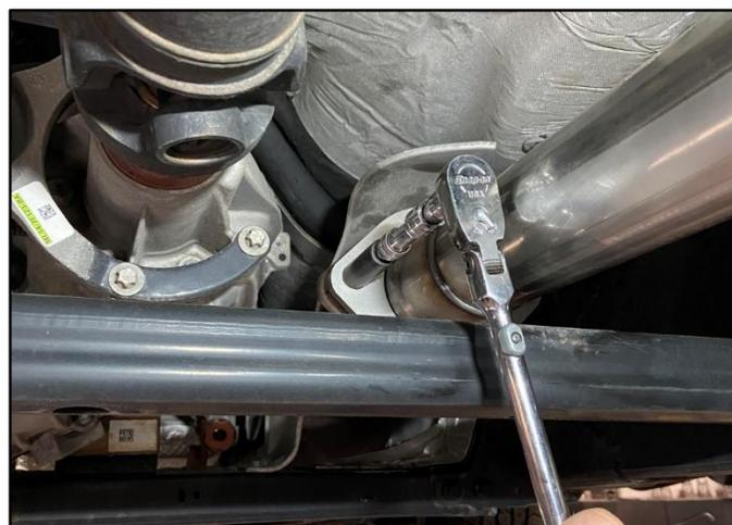
8. Locate the Head Flange Bolts from Removal Step 7. A second person may be needed to assist with this step.
