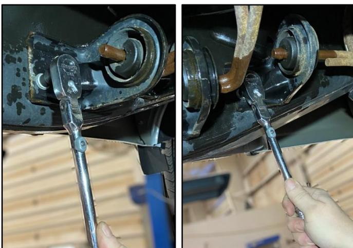
2. Use a 10mm Socket & Ratchet or Wrench to remove the 2 Bolts on each of the Factory Grommets. If the vehicle does not have the Flex Connector shown, the vehicle will have one Factory Grommet and may look different than shown.
