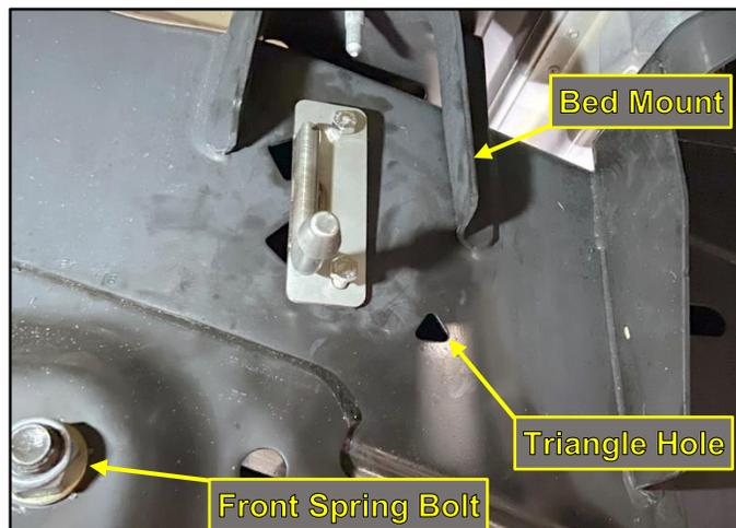
5. Locate the Frame Hanger and 5/16in Bolts in the Hardware Kit. Thread the 2 Bolts thru the Frame Hanger and into the Clip Nuts previously installed in Step 4.
