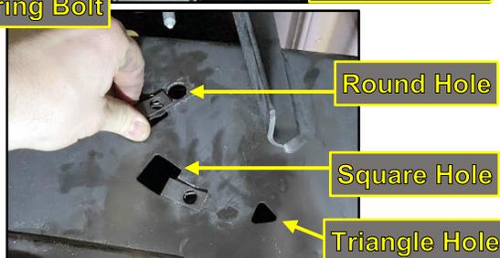
4. Insert the Clip Nuts into the Square Holes so the Nut is aligned with the Round Hole.
