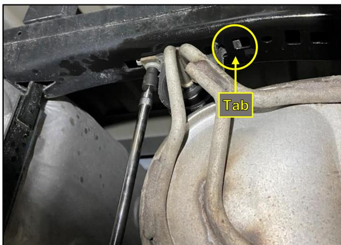
3. Locate the Middle Factory Grommets and use a 10mm Socket & Ratchet with an Extension or Wrench to remove the Bolt that attaches it to the Frame. Pull the Factory Grommet toward where the Bolt was attached. This releases a tab from a hole in the Frame.
