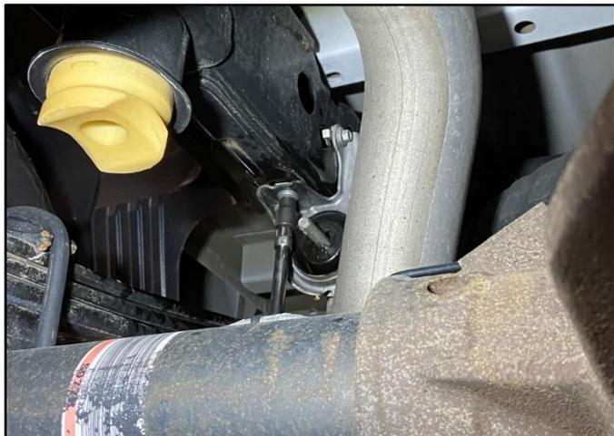
4. Above the Rear Axle, locate the Rear Factory Grommet and use a 10mm Socket & Ratchet with an Extension or Wrench to remove 1 the of bolts that attaches it to the Frame. One Bolt is vertical, on the bottom of the Frame. The other is on the inside of the Frame and is horizontal.
