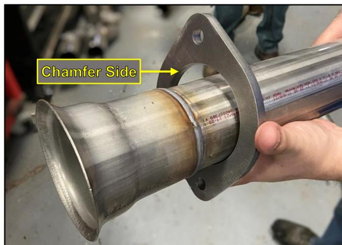
7. If installing a CORSA exhaust with a preassembled Head Pipe Flange on the muffler, skip to Step 10.
