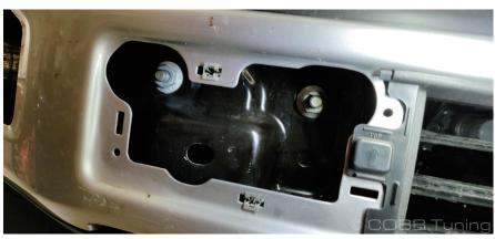
2. With a friend supporting the bumper, remove the 3 bolts on each side of the bumper using a 19mm socket and ratchet then remove the bumper and put it in a safe place.
