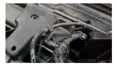
11. Remove the 4 8mm bolts holding the top part of the grille shell in place.
