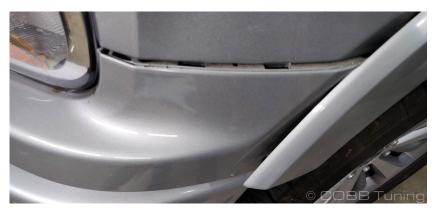
8. With the trim removed, use your 8mm to remove the 8mm bolts found on the lower right corner of each side underneath the headlight.
