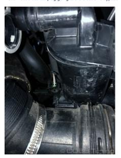
4. Loosen up the 3 couplers on the front mount intercooler, then pull them free. If you can manage it easily you can also just remove them completely. In order to loosen them you'll either need a screwdriver of a socket (7mm/8mm depending on your vehicle)
