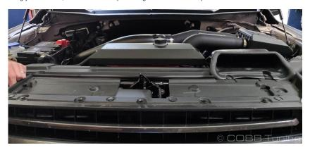
3. Remove the other seven clips holding the upper grill/radiator cover in place.
