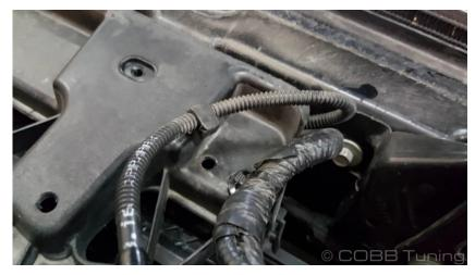
12. Remove the 4 8mm bolts holding the top part of the grille shell in place.
