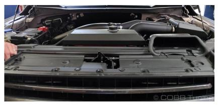
3. Remove the other seven clips holding the upper grill/radiator cover in place.
