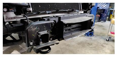
3. Unbolt the lower 8mm bolt on either side to remove the intercooler shroud from the car.
