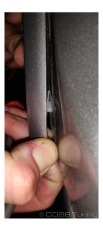
7. With both corners free firmly pull outward on the under-grille trim to remove it from the car. Set it somewhere safe.
