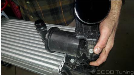
9. Take out the two lower bolts for intercooler shutters using an offset 8mm wrench. There isn't a lot of room so a ratcheting wrench with an offset head that fits can be handy, otherwise you'll be in for a long haul!
