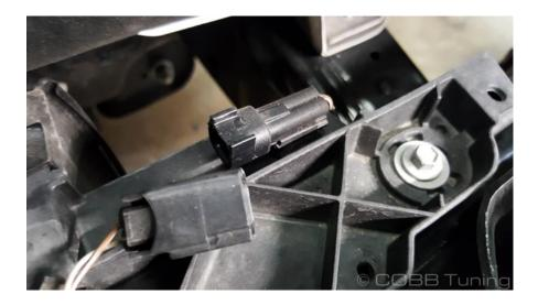
14. Remove shutter assembly by lifting up and pushing out to release the tension from the pins on the side
