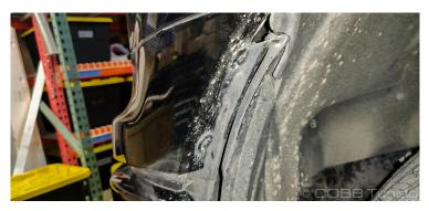
6. Gently pry outward on the fender flare and pop the clips free with your trim tool, making sure not to scratch the paint in the process (laying down painters tape on top of the paint can prevent minor scratches. (If not equipped with the fender flares skip this step.
