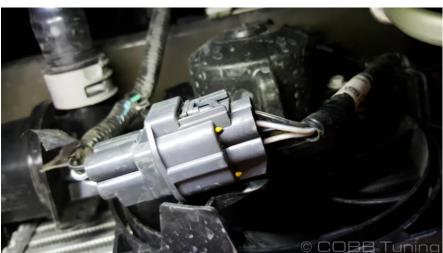
Disconnect electrical plug going to the electronic bypass valve.
