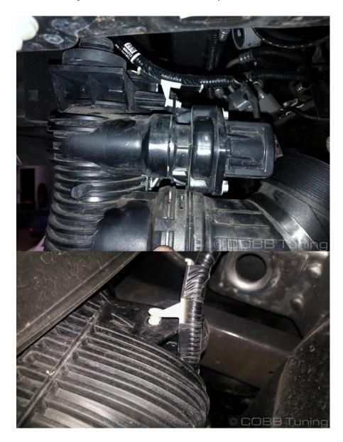
8. Drop the intercooler and fans out of the frame rails and set somewhere safe.
