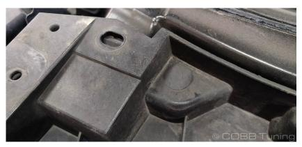
5. In the front corner of the wheelwell of the front two wheels you'll find two small 7mm bolts on the passenger's side, and either one or two on the driver's side. Remove them using your 7mm wrench.
