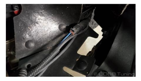
11. Undo the harness clips from shutter assembly so that the harness is free.
