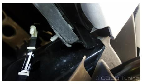
10. Disconnect the front 3 trim clips to pull up the rubber radiator shroud
