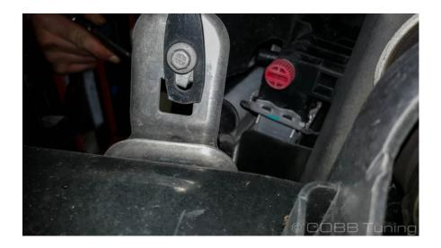
16. Follow up by taking out the 15mm bolts holding bracket in place
