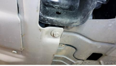
⚠ The clips with built in nuts found on the frame can fall off easily, so make sure not to lose them!
