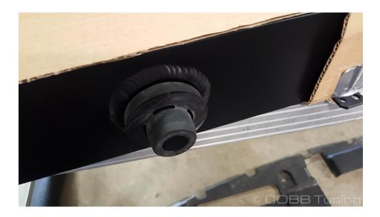
2. Remove your BPV from the intercooler core using an 8mm socket. Turn the BPV counter clockwise until it stops and then pull upward gently to remove.
