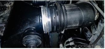
6. With the piping connected loosely, push the intercooler the rest of the way up into the mount, making sure that the rubber mounts sit inside the holes in the mount above. If your vehicle has the intercooler fans equipped, you'll want to tuck the top pins into the upper mount before pushing the intercooler all the way up as the fans fit around the intercooler in a "U" shape.
