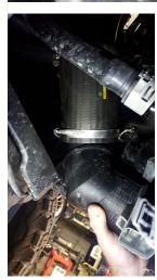
5. Disconnect the bpv hose from the intake and the BPV itself by turning left 1/4 turn. Sometimes it will be stuck due to dirt or debris getting into the clip. Softening it with some wd40 or water can make this more simple.
