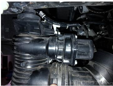
8. Drop the intercooler and fans out of the frame rails and set somewhere safe.
