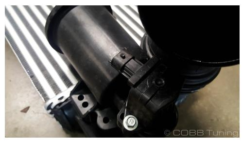
3. After checking to make sure the o-ring isn't torn. Lubricate the o-ring with super lube then Install the bpv by holding it at the shown angle and gently wiggling until it slides in, then turn clockwise until it stops
