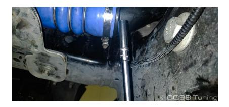
8. Reinstall the bottom intercooler mount
