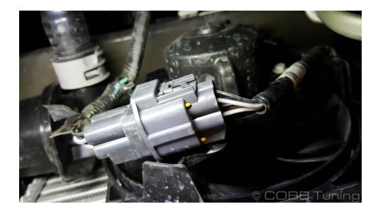
3. Disconnect electrical plug going to the electronic bypass valve.
