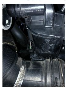
4. Loosen up the 3 couplers on the front mount intercooler, then pull them free. If you can manage it easily you can also just remove them completely. In order to loosen them you'll either need a screwdriver of a socket (7mm)
