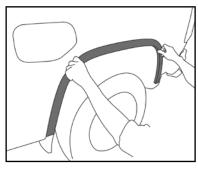
**STEP 2.** Firmly press Carrichs' fender trim onto vehicle's fender and mark reference points located on fender trim. Do this to all pilot holes on fender trim.
