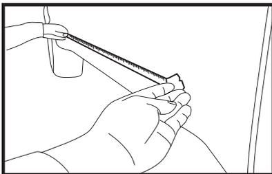
2. Determine location of where universal Body Side Moldings will be placed. Moldings must only be installed on a flat non curved section of the door to adhere properly. Only measure the flat non curved section of the door and determine if you have the correct length moldings before proceeding. Allow no more than 2 inches of clearance on each end of the Body Side Moldings to door edge for optimal clearance and appearance.
