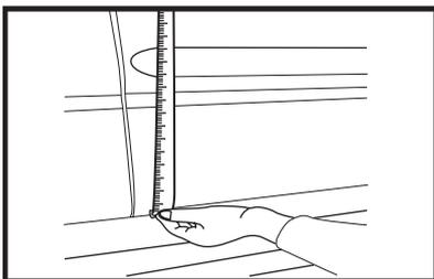
4. Confirming masking tape is straight and level. With tape measure, measure vertically along door. Lengths should be the same along both sides of tape. Use horizontal centerline of each molding piece. If heights are different make adjustments until they are equal in length.
