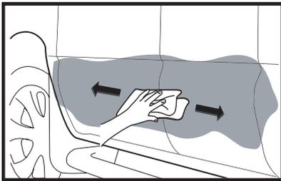
1. Wipe down surface with a soft towel soaked with alcohol to remove any wax or contaminants from paint finish of vehicle's lower door area.
