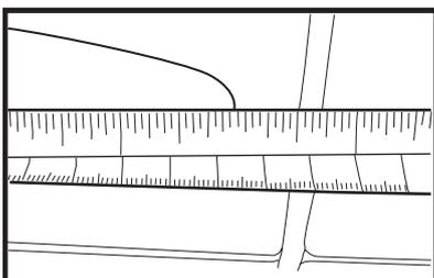
5. Place Body Side Moldings on vehicle's door. Body Side Moldings should have 2 inches clearance between door edges to allow door to fully open without impacting Body Side Moldings. Start at one end of the door and work your way to the other side using masking tape as guide to insure straight and even installation. Once Body Side Moldings has been installed and leveled, press and hold molding down against door for 10 seconds for proper bond.
