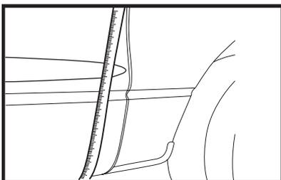
3. After confirming you have the correct length moldings, mask off a straight section on the door to use as a guide to aid in installing the moldings straight and level. Take into consideration clearance needed to open door. (2 inches)
