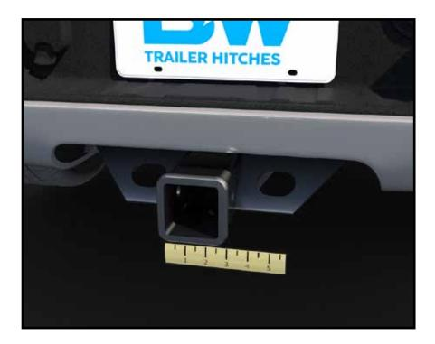
Remove any reducer sleeves (smaller tubes) from the receiver tube and measure the opening as shown. Using reducer sleeves can decrease the tow rating of your hitch and create additional noise while towing.
