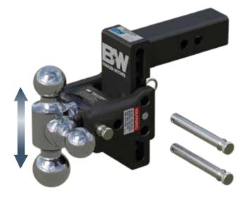
Along with proper weight distribution of the cargo and staying away from loads that exceed the capacity of the trailer, keeping your trailer level helps to maintain good handling characteristics while driving. Keeping your trailer level may mean using your Tow & Stow in an inverted position. When you need more rise for the ball, simply turn the Tow & Stow upside down in the receiver socket.
