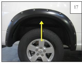
Start supplied screw (SW1-0056) using a Phillips screwdriver. *Do not tighten*.
