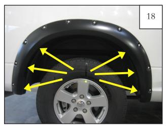
Hold flare to vehicle and start re-installing the (6) factory screws with a 8mm socket. (Part number 50937 uses (5) screws only.) *Do not tighten*.
