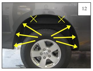
Remove these (6) factory installed screws using an 8mm socket wrench. X's indicate a factory screw that will not be removed. Retain screws to be re-used to install the rear flare. (Part number 50937 uses (5) screws only.)
