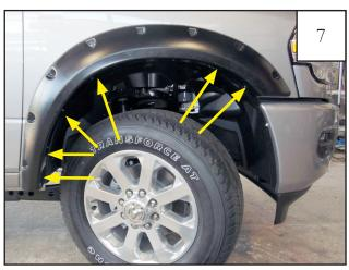
Hold flare to vehicle and start re-installing the (6) factory screws with a 8mm socket. *Do not tighten*.
