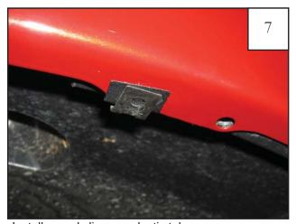
Install speed clip over plastic tab.
