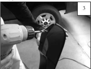
**OPTIONAL BUMPER PIECE:** Using a 5/16" drill bit, drill two holes in dimpled hole locations for both flare and bumper piece. Note: Holes only need to be drilled if bumper piece is being used.
