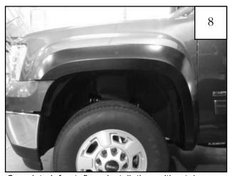
Completed front flare installation without bumper piece.
