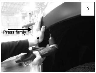
Check that flare is positioned correctly around wheel well. If not, adjust before tightening screws. Then, making sure bumper piece and flare seams are still aligned with factory seams, *firmly* press the flare up and toward the vehicle while tightening all screws.
