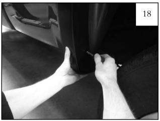
Start a supplied Screw (SW1-0050) through each of the remaining holes and into each Clip installed in Step 16. If needed, use scratch awl (or similar pointed tool) to locate holes. Tighten all screws.
