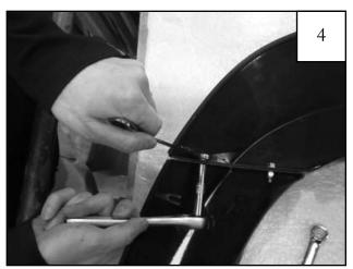
**OPTIONAL BUMPER PIECE:** Using 3/8" and 7/16" wrenches, attach bumper piece to flare using supplied Screw (SW1-0005) and Nut (NU1-0015). Make sure both pieces are properly aligned before tightening. *NOTE: Do not overtighten or parts will warp.*
