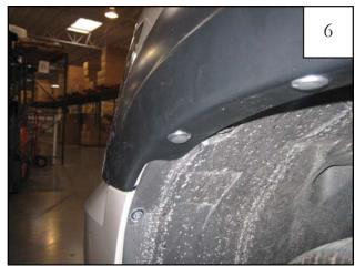
Install a supplided Retainer (RV1-P006) through hole drill in Step 5.
