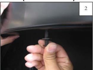
Holding flare in position on fender, install two supplied plastic Retainers (RV1-0006).
