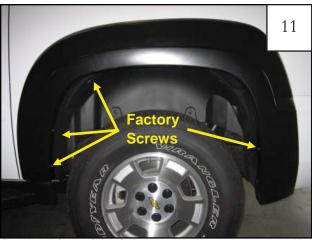
Reinstall four of the five screws that were removed in Step 8, into the locations shown.
