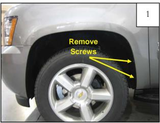
Using a 9/32" socket, remove two factory screws. Retain screws for later use.
