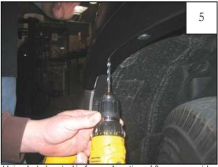
Using hole located in forward portion of flare as a guide, drill through the splash sheild with a 5/16" bit. Holes in flare and splash sheild should align with factory hole located in fender.
