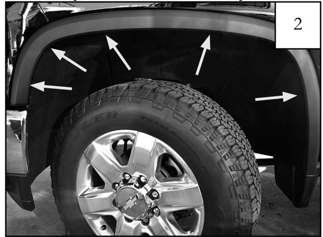
Remove (5) factory installed screws.
