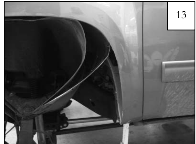
Bend inner fender metal away from fender.
