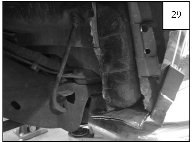
Cut pinch seam at mark made in previous step. Bend flange inward even with firewall.
