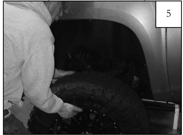
Support vehicle and remove tire.
