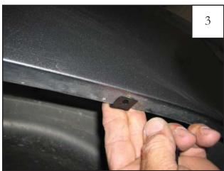
Slide a supplied Plastic Clip over two top marks made in Step 1. Clips may need to be adjusted to align with holes in flare. *NOTE: the raised collar on the clip should face upward into the interior of the fender.*
