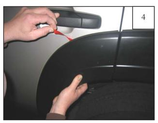
Confirm placement of the part. Gently pull the tape liner from the tape, starting with the top tab you created.
