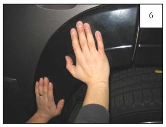
Apply firm pressure to taped areas for proper bond. Tape reaches maximum adhesive bond after 24 hours of contact. Do not wash vehicle until 24 hours have passed.
