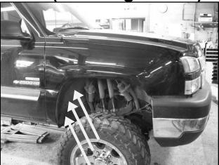
Remove three factory fasteners from the inner splash shield. Save factory fasteners for reinstallation.
