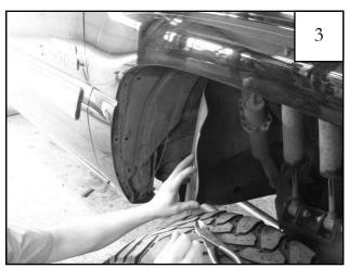
Pull splash shield forward out of the way of the wheel well.
