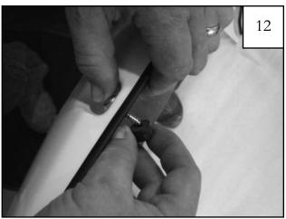
Install a supplied Screw (SW1-0045) through each pocket hole in flare and thread a Spacer (SP1-0009) over the end.
