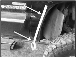
Run a piece of masking tape vertically from 0" at body line to 1.25" mark made in previous step.
