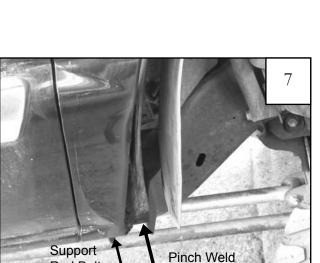
Once the sheet metal is removed, take a hammer and roll over 5.5" of the bottom of the pinch seam of the cab and any inner fender. Deburr edges and seal with primer. Remove bedside support rod bolt at lower rear of the wheel well. Reinstall splash shield using factory hardware.
