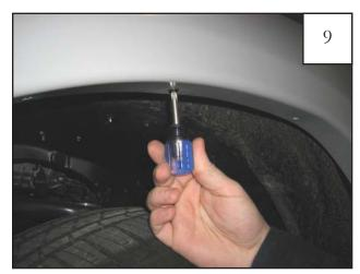
Replace flare on fender, aligning holes with holes in clips. Start three supplied Serrated-Flange Screws through three holes in flare and into "S" Clips installed in Step 7.
