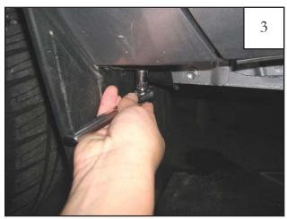
Remove screw from underside of factory mud guard. Note: If vehicle is equipped with running boards, running boards may need to be removed in order to access this screw.
