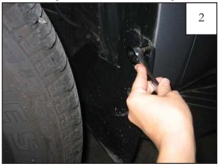
Using a socket wrench with a 10mm socket, remove top screw from factory mud guard as shown.
