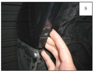
Slide a supplied "U" Clip over the fender lip, aligning with forward-most hole in fender. Note: For the Limited version, skip this step.
