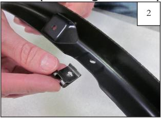
Verify 3 "U"clips installed on the inner bracket as shown. If they are not installed, attach 3 "U"clips (CL1-0022) to the inner bracket as shown.
