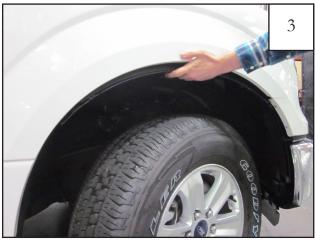
Line up the holes in the inner piece with the three uppermost factory holes. NOTE: Driver's side inner piece is marked with an "LH" and passenger's side inner piece is marked with an "RH".
